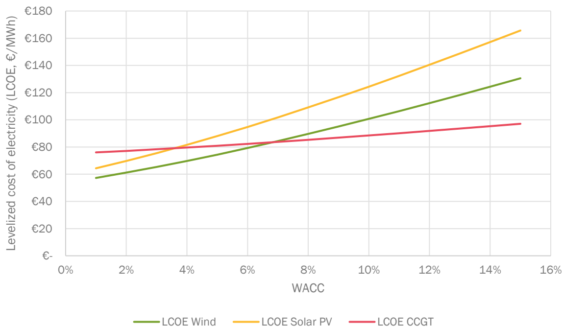
Figure 4: Levelized cost of electricity, as a function of the WACC, for three selected technologies
